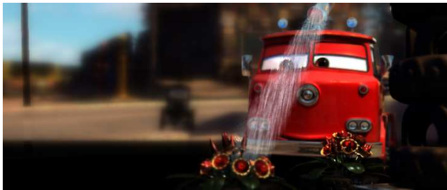
Figure 1: Top: Pinhole camera image from an upcoming feature film. Bottom: Sample results of our depth-of-field algorithm based on simulated diffusion. We generate these results from a single color and depth value per pixel, and the above images render at 23–25 frames per second. The method is designed to produce film-preview quality at interactive rates on a GPU. Fast preview should allow greater artistic control of depth-of-field effects.
