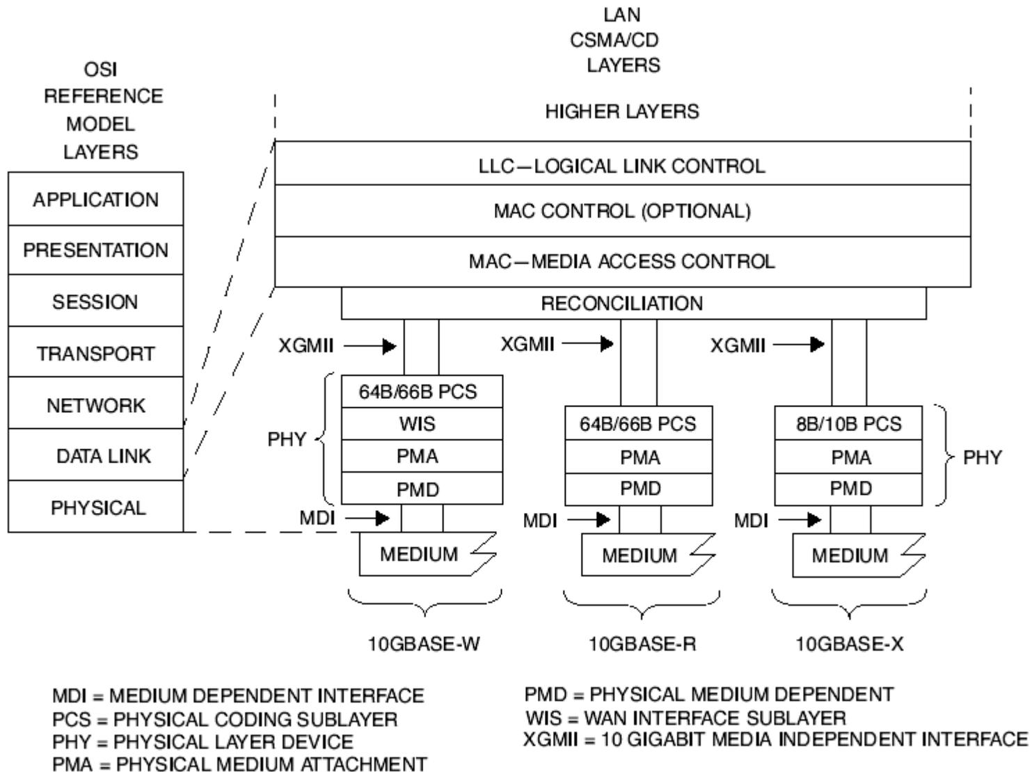
**Figure 44-1 – Architectural positioning of 10 Gigabit Ethernet**
