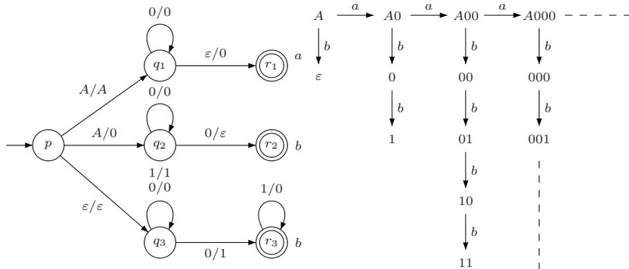
The encoding of the vertices of this tree relies on the fact that there are  $2^n$   $n$ -tuples over  $\{0, 1\}$ . The transducer performs the binary addition.
