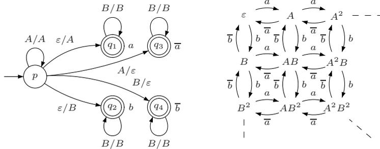
We simulate two counters machines on the unfolding of this graph. As these machines may test for zero, we add a loop on each vertex expressing that either counter, both or none is empty (denoted respectively by  $\#_a, \#_b, \#_{ab}, \#$ ).
