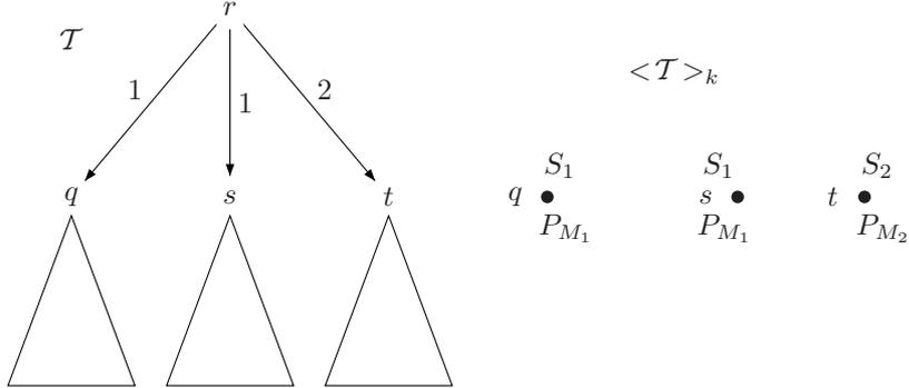
The tree depicted on the left is defined over  $\Sigma = \{E_1, E_2\}$ , the reduced tree  $\langle \mathcal{T} \rangle_k$  is defined over  $\langle \Sigma \rangle_k := \{S_1, S_2\} \cup \{P_M \mid M \in \text{Thm}_k^\Sigma\}$ ; and  $\text{Thm}_k(\mathcal{T}_q) = \text{Thm}_k(\mathcal{T}_s) = M_1, \text{Thm}_k(\mathcal{T}_t) = M_2$
