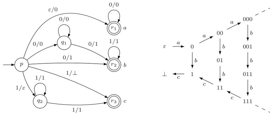
The path  $p \xrightarrow{0/0} q_1 \xrightarrow{0/1} r_2 \xrightarrow{1/1} r_2$  accepts the couple  $(001, 011)$ , the final state  $r_2$  is labelled by  $b$  thus there is a arc  $001 \xrightarrow{b} 011$  in the graph.
