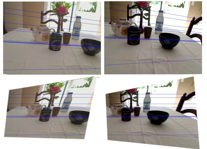
Fig. 2: Rectified image pair using Hartley [3] : the epipolar lines are horizontal and aligned from an image to the other. The rectified images are suited for computer vision processing, but not for stereoscopic rendering.
